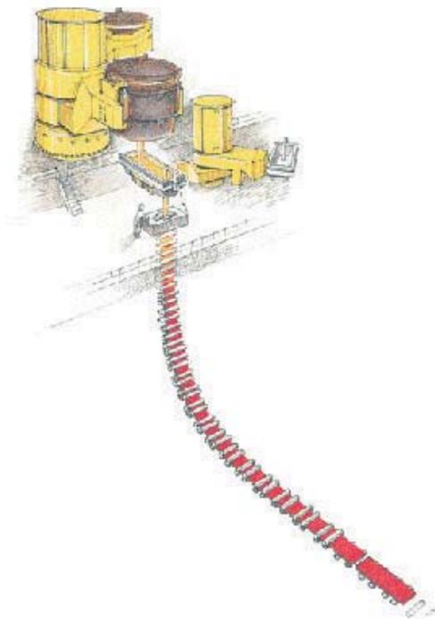
which one is in use and the other is being re-surfaced. The repair of the rollers is either carried out by an individual unit of the steel plant or by a dedicated external company. Soft martensitic weld metals are commonly used as an alloy for surface welding. They consist of approx. 13% chrome, 4% nickel and about 1% molybdenum. These alloys have been a great success because of their combination of resistance to heat, thermal shock, corrosion and wear.
