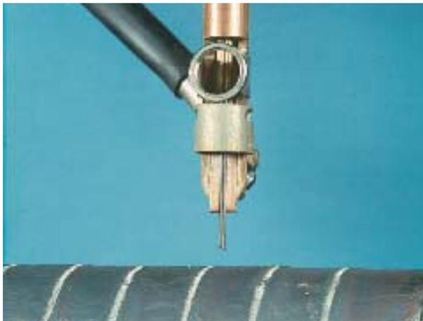
Fig. 4. Sub-arc cored wire surface welding with OK
